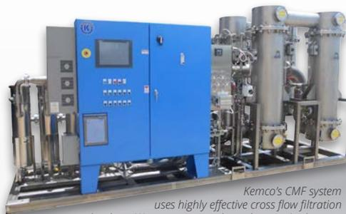
*Kemco's CMF system uses highly effective cross flow filtration technology. Wastewater runs through ceramic elements in the filter modules, passing through pores in the filter element, to produce a product water filtrate. Cleaned filtrate is diverted to a storage system for recycling and contaminants are removed in a small concentrate stream.*
