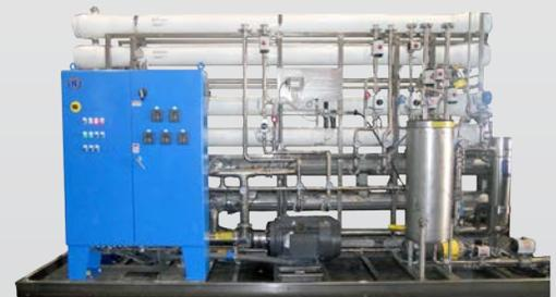
*Reverse Osmosis added after Ceramic Microfiltration increases recycle rate and TDS levels of the permeate are less than 300 ppm.*
